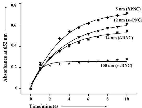
**Figure 2.** Nanoceria-promoted oxidation of TMB is size-dependent. At pH 4.0, smaller ceria nanoparticles show higher oxidase-like activity than larger nanoparticles.
